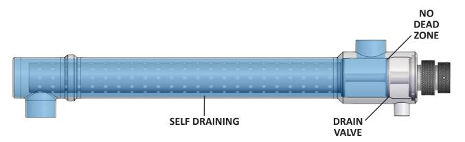
Within the main body size, the internal design of the Housing and SafeLock mechanism is always the same. The filter inserts are exchangeable. The filter insert specification can vary greatly (5um to 5mm).
