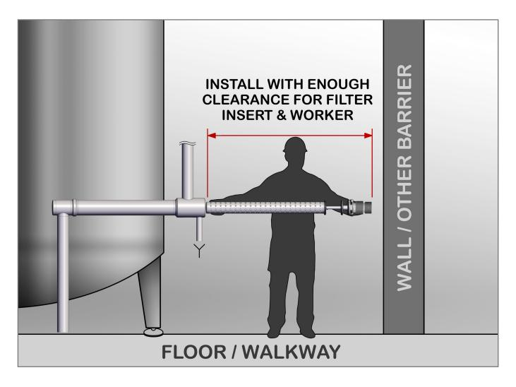
4. On defaullt, the **SafeStrainer** is installed horizontally so that the housing empties completely when the drain valve is opened. All installation directions are possible for pressure relief. However, the **SafeStrainer** can be installed in every possible position and safe operation is ensured if the instructions above are followed.
