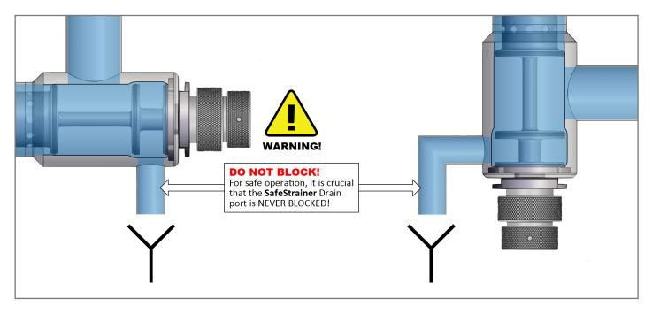
2. If the operator cannot see the end of the drain pipe, it is recommended to install a sight glass in the drain pipe so that the operator can ensure that the entire pipe system is completely emptied before opening the Safe Lock Disc by turning the Safe Lock Handle (as shown in Step 2 of **3.1 Removing the Filter Insert** on page 19).
