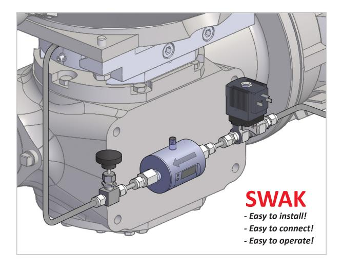
SWAK is a device that ensures proper supply of seal water for double acting mechanical seals (DAMS). It can be installed on any machinery that is equipped with DAMS such as agitators, pumps, mixers, and emulsifiers.
