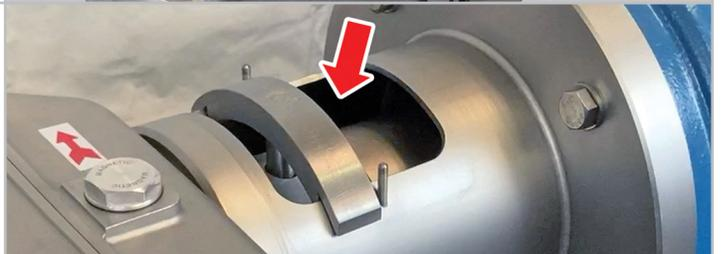
The exchange of the mechanical seals in a **ViscoTwin G10** is safe, fast and secure. All pins and alignment plates are eliminated. The cartridge design makes it a simple one-piece exchange process.
