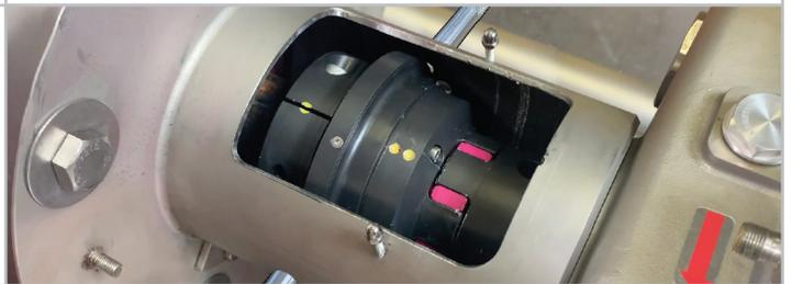
With the gapping port the service technician can tune the shafts in 10 minutes. No pump parts have to be disassembled and no gear oil needs to be released.
