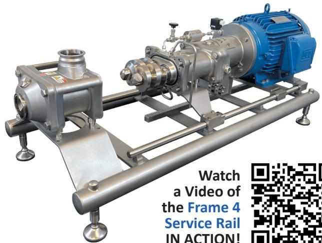
In case a piece of foreign matter enters the pump and blocks the spindles, the dis-engaging coupling protects the pump head from severe damage.
