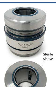
With Huhnseal AB in Sweden we designed **ViscoTwin G10** cartridge seals that are easy and reliable to install. All pins and bolts are now eliminated. The stators are positioned with "flats". The seals are pressed in position by hand.
