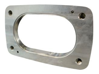
The **WELD-IN FLANGE** allows for close-coupled installation of the pump to a tank or auger in case the product is too viscous to flow through a valve and pipe into the pump. The Weld-In Flange is available for customized installation with the matching weld in jig.
