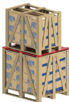
Figure 28 - Use of additional battens for stacking
