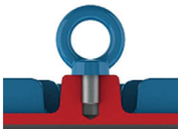
Figure 4 - Correct tightening of the eyebolt
