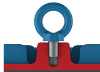
Figure 5 - Incorrect tightening of the eyebolt
