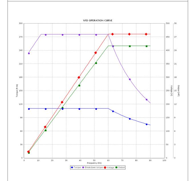
Performance : 460 V 60 Hz 6P : 30.4 A Moment of inertia (J) : 11.5 sq.ft.lb Rated current LRC : 6.0 Duty cycle : Cont.(S1) : 110 ft.lb Insulation class : F Rated torque Locked rotor torque : 210 % Service factor : 1.25 Breakdown torque : 250 % Temperature rise : 80 K Rated speed : 1175 rpm Design : B
