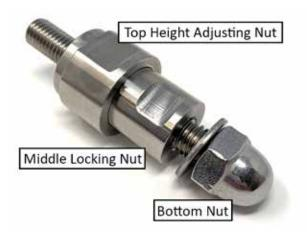
4. Adjust the THREE (3) adjacent Alignment Adjusters in the same fashion, and once the desired positioning has been achieved, tighten the **Bottom Nuts** on the Alignment Adjuster Bolts up against the bottom surface of the support bracket.
