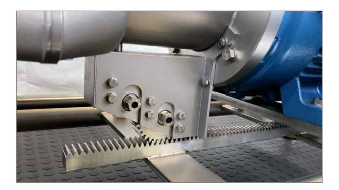
Frame #4 is OPENED and CLOSED by using a 19mm socket wrench (with extender) on the small gear drive wheel of the Gear Box, from either side of the pump. While the larger gear wheel can also be turned to move the assembled Pump and Motor on the sliders, it is recommended to use the Small Gear Wheel for more precise control.
