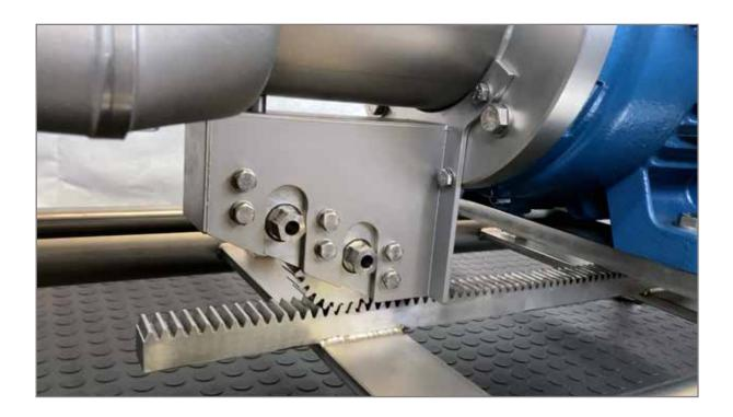
Frame #4 is OPENED and CLOSED by using a 19mm socket wrench (with extender) on the small gear drive wheel of the Gear Box, from either side of the pump. While the larger gear wheel can also be turned to move the assembled Pump and Motor on the sliders, it is recommended to use the Small Gear Wheel for more precise control.
