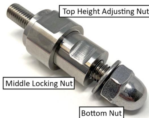
**NOTE:** The **Middle Locking Nut** is designed to be extra tall in order to cover the exposed threads of the bolt between the **Top Height Adjusting Nut** and **Middle Locking Nut**.
